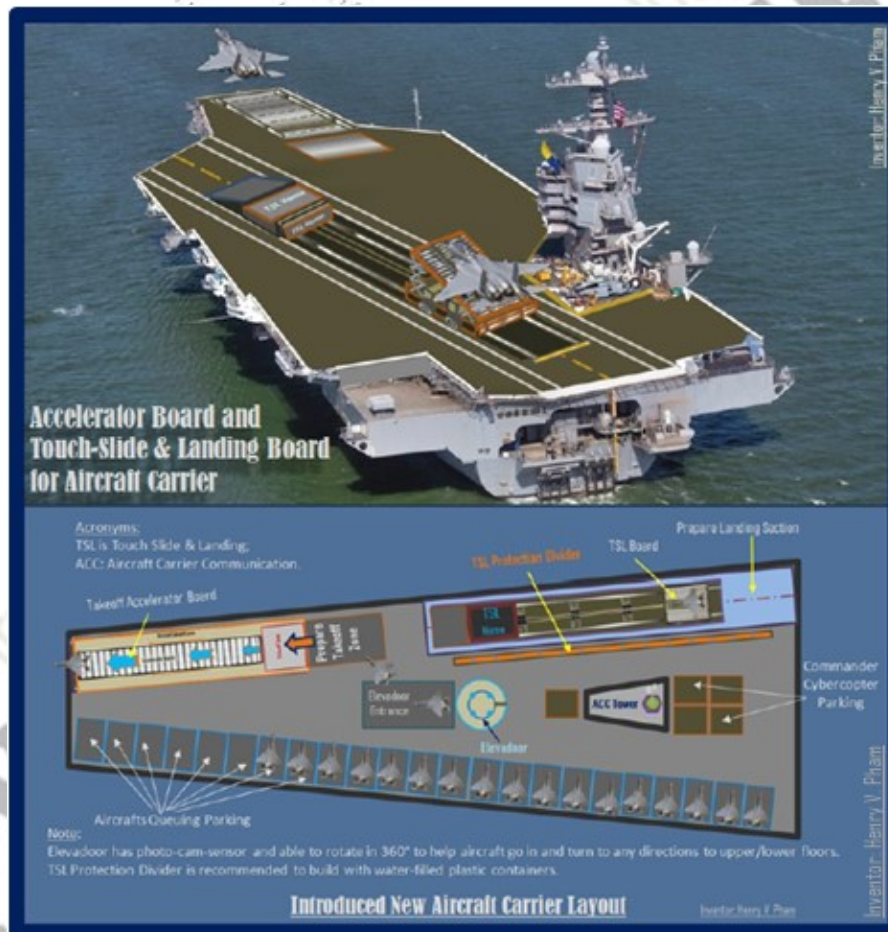
Figure-A: Touch-Slide & Landing Board for Aircraft Carrier -- Overview
